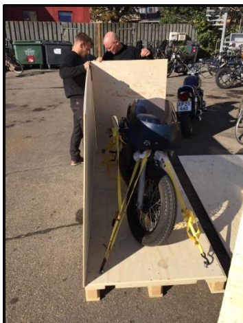
The box is built up around the motorbike. Smooth surface of the boxes, no nails and customized locking system ensure safety of motorbikes while they are in transport .
