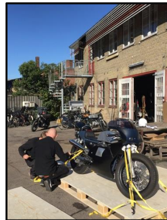
The hooks at the sides of the wooden panel keep the motorbikes stable through strapping.
